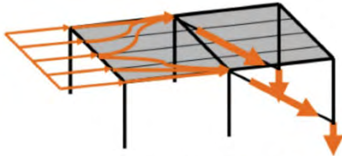
Load Path for a Lateral System
