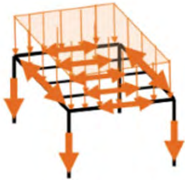
Load Path for a Gravity System
