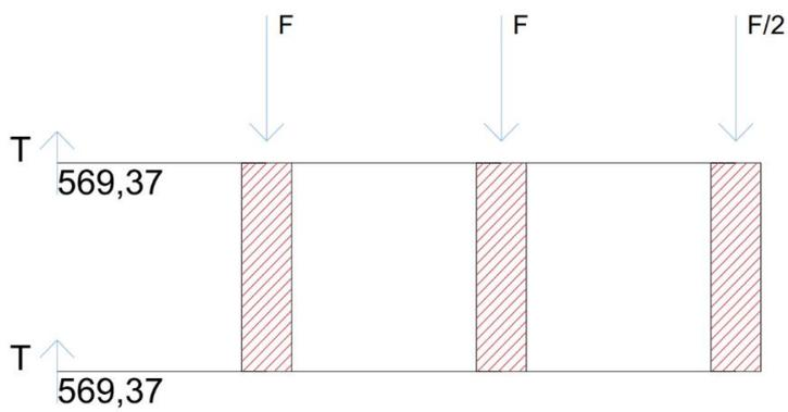
Trave IV:  $2T = F + F + F + F/2 \rightarrow 7/4 F \quad T = 797,12 \text{ Kn}$
