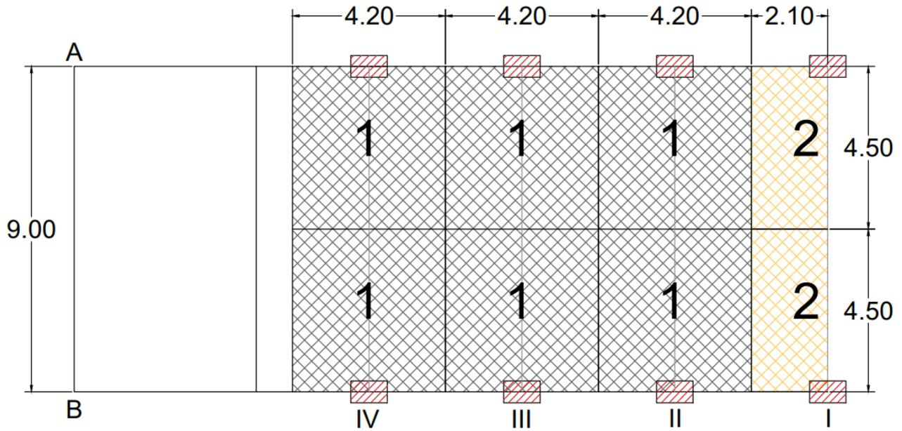
$Q_s = 3,5 \text{ Kn/m}^2$      $Q_a = 2,00 \text{ Kn/m}^2$      $Q_p = 3,0 \text{ Kn/m}^2$      $Q_u = 12,05 \text{ Kn/m}^2$
