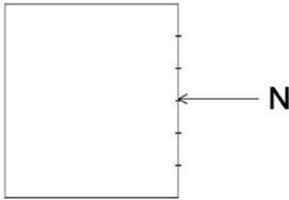
$$e = \frac{M}{N} = 4,37 \text{ mm} < \frac{H}{6} (75 \text{ mm}) \quad \text{CASO I}$$
